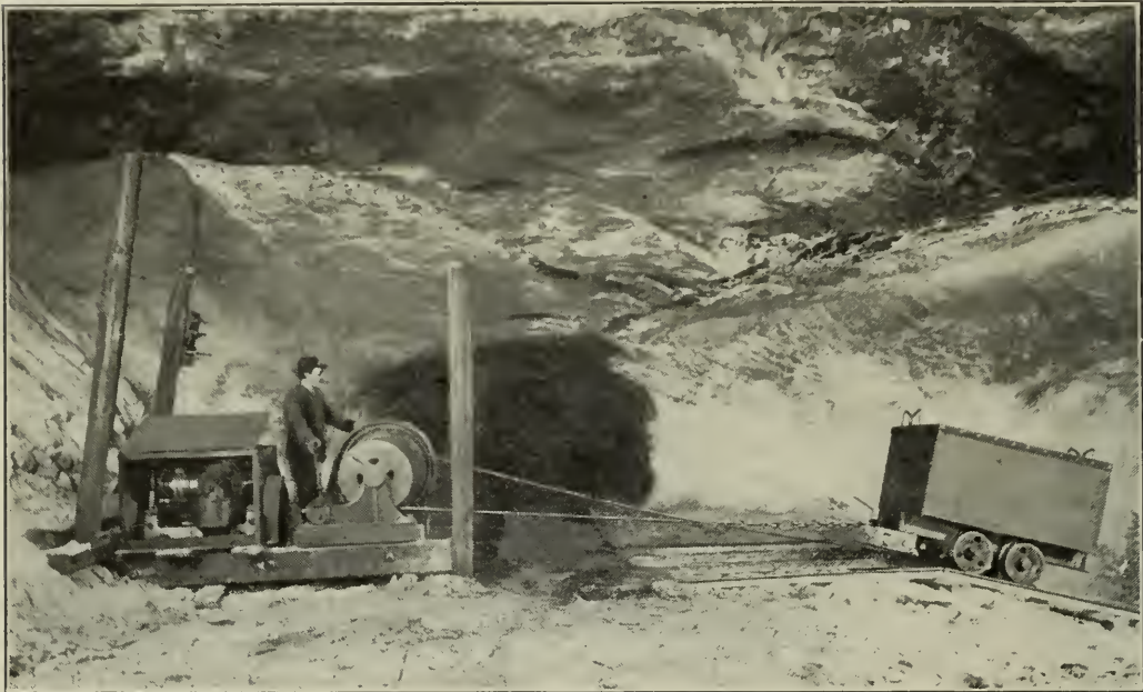
FIG. 22. HAULAGE BY ELECTRIC MOTOR, MINES OF THE KALIWERKE ASCHERSLEBEN. burg (South Africa), Shimoyamada (Japan) etc. have Siemens & Halske equipment; Schücker installed the plant at the Zwickauer Steinkohlenbau Vereins, the Altgemeinde Bockwa, etc.; Gans furnished electric haulage machinery for the mines of Kivald, Tokod, Resicza, Nagy-Manyok, and many other workings.
